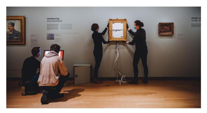
The museum is collaborating with ASML to develop a method to monitor paintings individually. This is a test setup fitted with 45 sensors that measure temperature, relative moisture and light.
